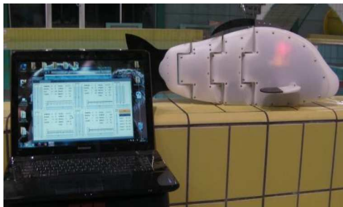
Fig. 2. Technology demonstrator for a bio-mimetic underwater vehicle with harmonic drive.
