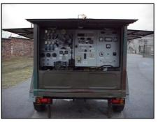
Fig. 6. Air supply system of the underwater works securing base "ORTOLAN" – control panel.
