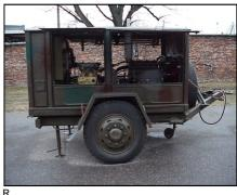
Fig. 7. The supply system for underwater works security base "ORTOLAN" with diving air compressors EK 2-150 manufactured by the former USSR
