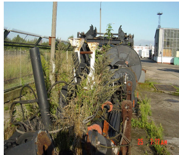
Fig. 8 The condition of the Af-2 system components of the chamber and bell lifting and lowering device in August 2003.
