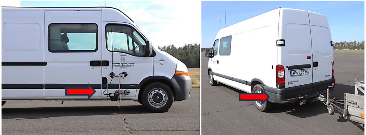
Fig. 9. View of measuring equipment used for the measurement of braking distance: Correvit S400 head on the left, Shot Marker on the right.
