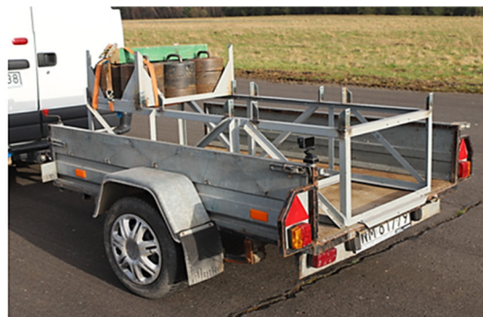
Fig. 5. View of a trailer loaded according to variant IV with an indication of the position of the centre of mass.
